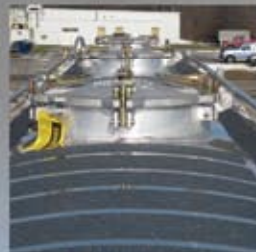
Manholes - Toe Rails
