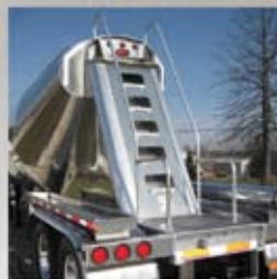
Double Hand Rails Enclosed Man Ladder
